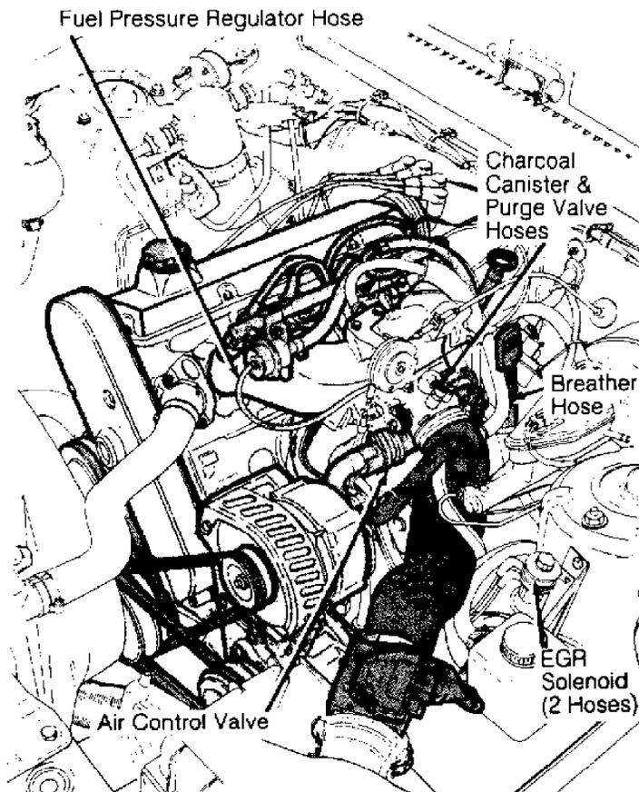
Fig. 1: Identifying Vacuum Hose System Components (940 Turbo)
