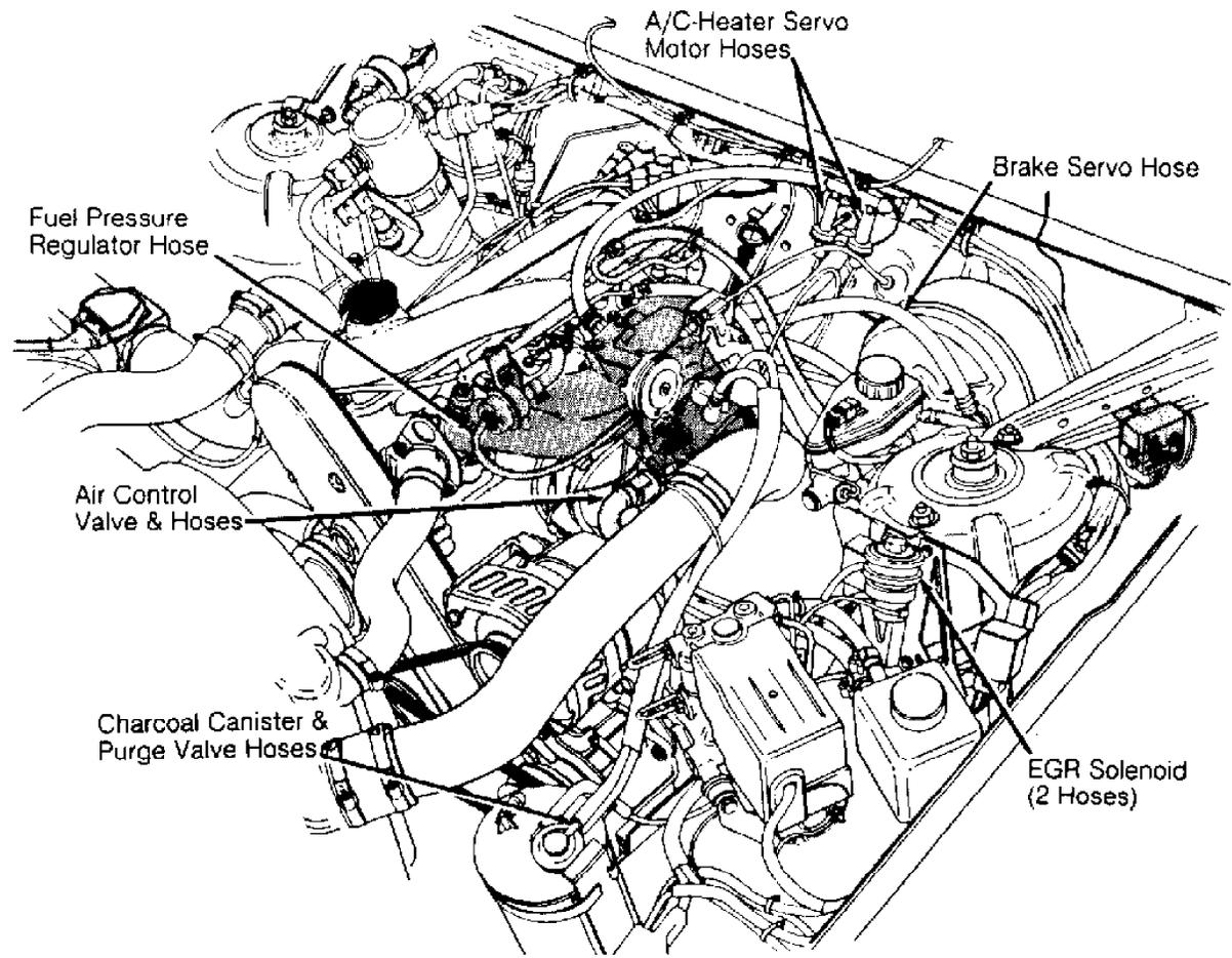
Fig. 2: Identifying Vacuum Hose System Components
