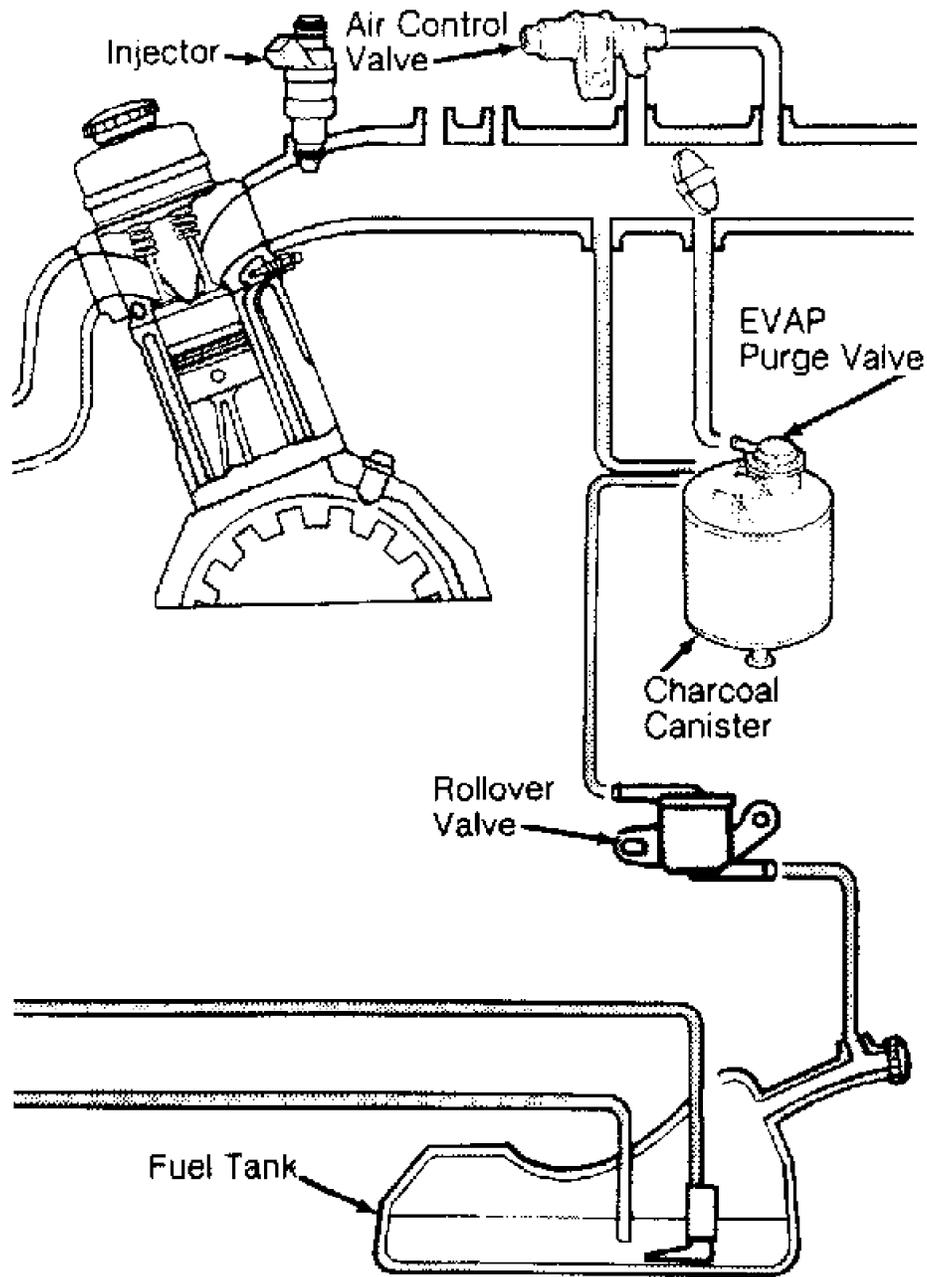
Fig. 3: Identifying Typical EVAP System Components (940)
