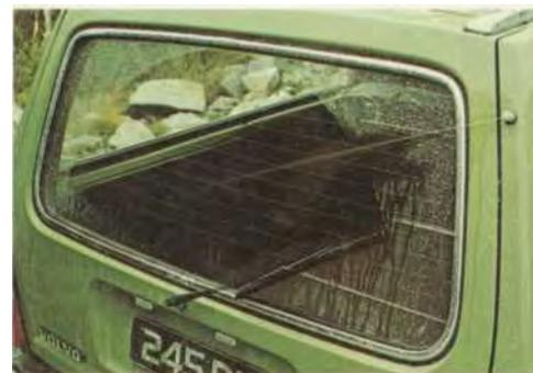
The new Volvo 245 tailgate window is electrically heated and has a wiper and washer as standard.
