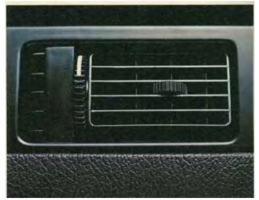
The new air nozzles serving the side windows are fixed, as their job is to keep the side windows clear at all times without any help from the driver.
