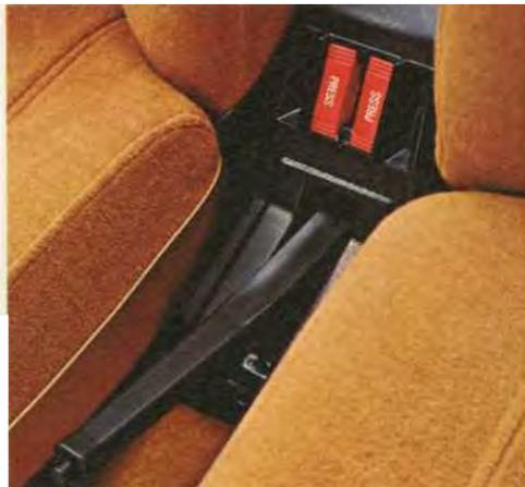
The handbrake is now located between the front seats in a housing which also incorporates the safety belt locks which are easier to use and easier to see, even at night, since they are illuminated.
