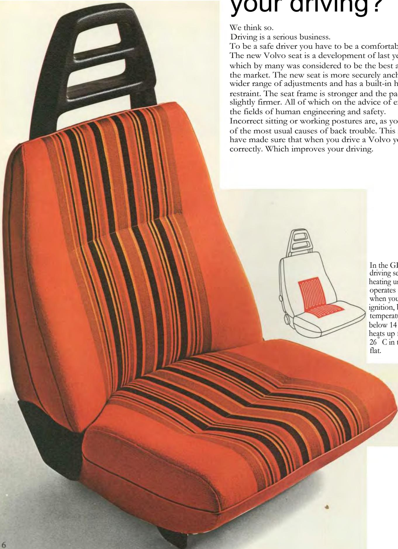
In the GL model, the driving seat incorporates a heating unit. The element operates automatically when you switch on the ignition, but only if the temperature in the car is below 14° C. The seat heats up from 0° to 26° C in three minutes flat.
