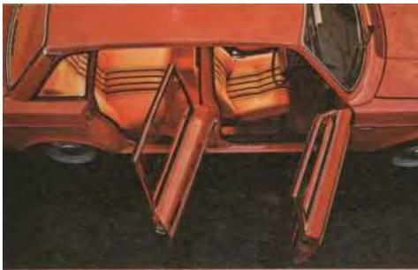
Wide opening doors - no less than  $80^\circ$  - allow convenient, and dignified, entry and exit. Each door incorporates a strong tubular member to protect you and your passengers from side impact.
