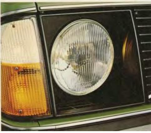
The halogen headlights are bigger for safer night driving.
