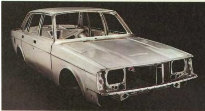
Volvo's already famous rust-proofing has been improved still further on the 1975 Volvos. The number of galvanized metal pressings in the body has been increased, and now includes the wheel and spring strut housings. And then the entire body is submerged in an electrically-charged bath of primer. On top of that, we add the paintwork which makes you wish sunny Sunday mornings came more often.
