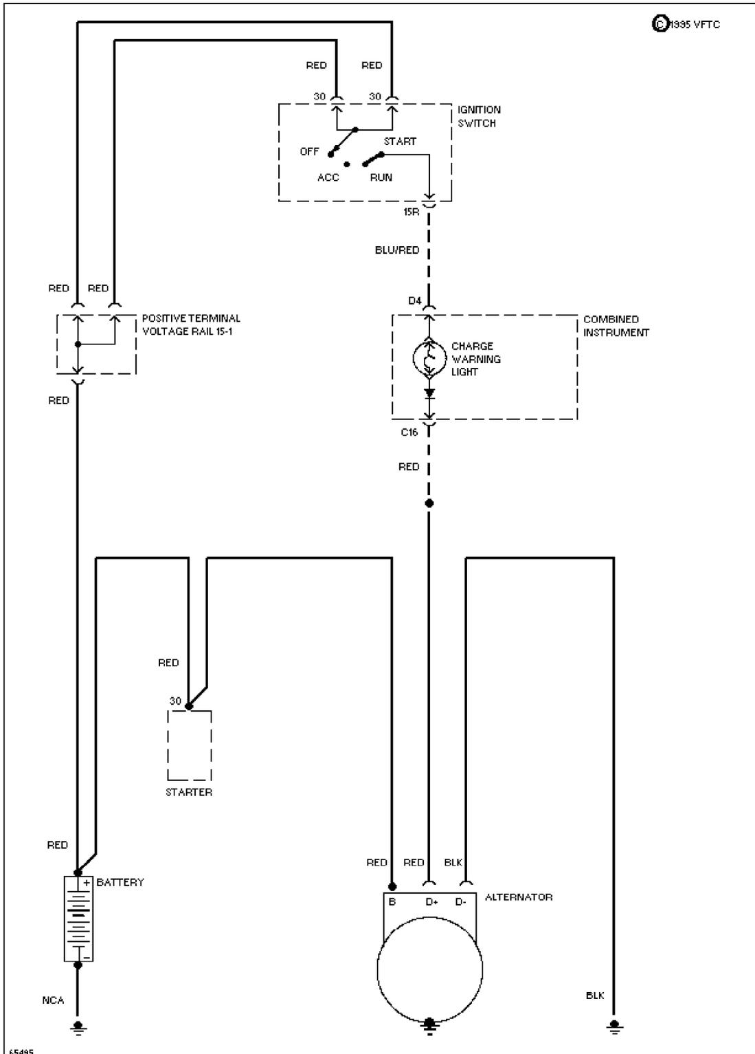
Fig. 3: Charging System Wiring Diagram (960)
