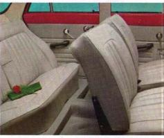
The front seat backrests on all models are easily adjusted into three positions. In the middle position on the two-door model, the backrests can be folded down to permit unobstructed passage to the rear seat. In the forward and rear positions, the seats are locked in position for safety.
