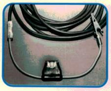
During testing, some guys prefer to run the fuel pump directly off the battery. To make a good jumper, splice a fuseholder and 10-amp fuse onto some 12-gauge wire. Be sure you have an alligator clip that fits the fuel pump terminal and another one that fits the battery terminal.
