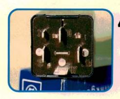
In order to run the fuel pump during your K-Jet tests, you can by-pass the fuel pump relay. See how the middle two terminals (30 and 87) form an inverted T? After you pull out the relay, just remember to connect your jumper wire across the two female terminals that form the T.
