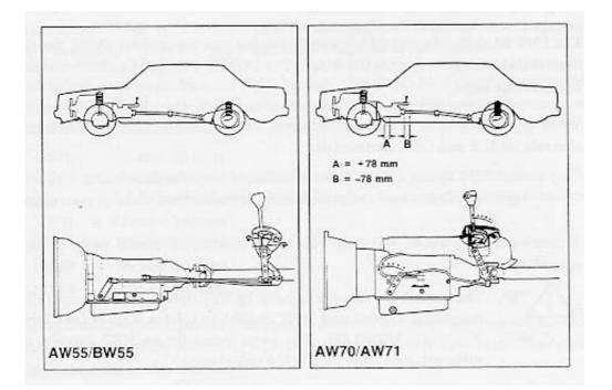
The AW70/71 transmissions are improved versions of the earlier automatics. The AW70 was fitted to normally aspirated (non-Turbo) four-cylinder sedans and wagons. The AW71 was fitted to all Turbo models equipped with automatic transmissions. The information plate on the side of the transmission and the VIC plate will positively identify the transmission.
