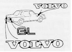
The letter designations provide only part of the info you need. Make your job easier by always getting at least the VIN. Letters can be tricky. For instances a 1980-81 GL is a 260 model -- a 1983-84 GL is a 240 model. Also, a few 1982 GLT models are NOT equipped with a Turbo engine -some in the United States have a B-21F, some in Canada have the B-23E!
