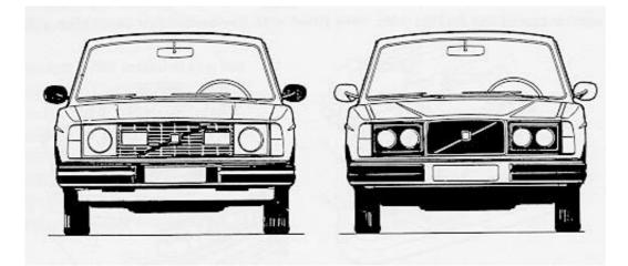
The headlamps were single round, dual round and dual rectangular headlight bulbs (the bulbs were called "inserts"). Although headlight inserts are listed by VIN on your Volvo Parts Manager's list, we have simplified things with the list below:
