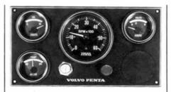
double fuses and switch for instrument lighting. Automatic main fuses with reset button. Extension cable, length 7 m, with plug-in connector fitted.
