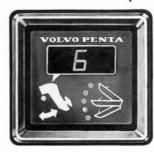
The trim angle is indicated by five green diode lamps plus a digital display. A continuous red light indicates when the drive is in the "beach" sector. The red light flashes when the drive is in the "tilt" position.
