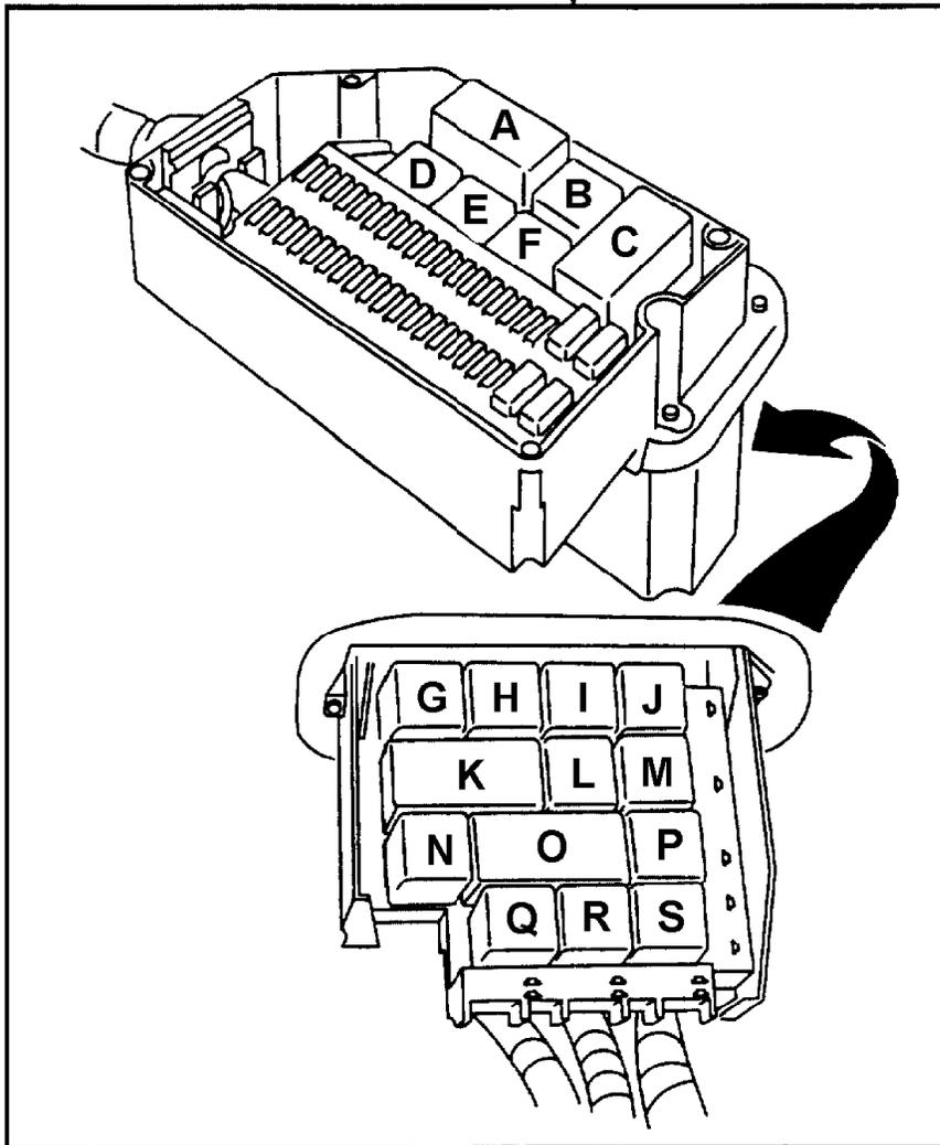
Fig. 2: Relay Panel Identification
