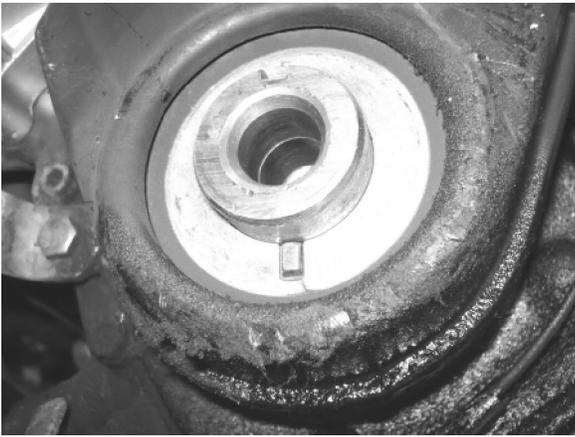
**Figure 11.** With the crankshaft pulley off, the front crankshaft shim and crankshaft end are exposed. (Note the oily residue at bottom of photo, which indicates a leaky crankshaft seal.)
