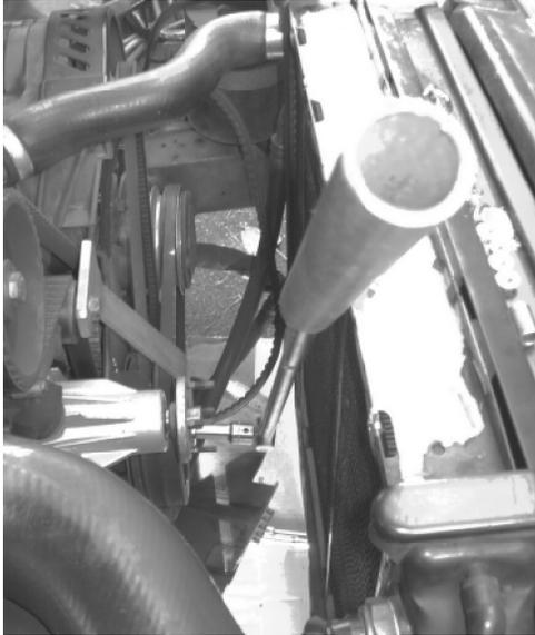
**Figure 8.** Use a long-handled wrench with a cheater bar (iron pipe) and 24 mm socket to break free (counterclockwise) the crankshaft bolt. Remove the bolt.
