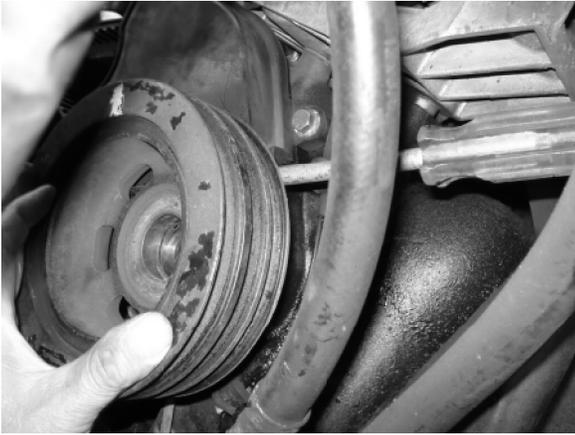
**Figure 10.** Without the belt tension, the crankshaft pulley should be easy to remove. Grab the pulley on opposite sides with both hands and rock it back and forth while pulling. If it is difficult to get off, gently pry in back with a flat-bladed screwdriver.
