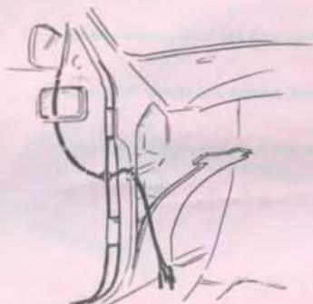
Run the cable through the existing rubber grommets in the door and A-post into the coupé.
