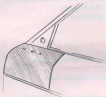
Place the template on the front edge of the door and mark where the holes are to be drilled.
