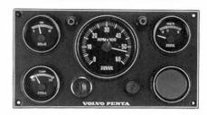
(Extra equipment for some markets.) Fitted with key switch, tachometer, oil pressure gauge, voltmeter, temperature gauge, double fuses and switch for instrument lighting. Cable length 6.0 m (19.7 ft).
