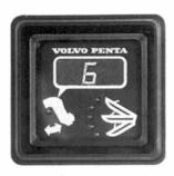
The trim angle is indicated by five green diode lamps plus a digital display. A continuous red light indicates when the drive is in the "beach" sector. The red light flashes when the drive is in the "tilt" position. The con-
