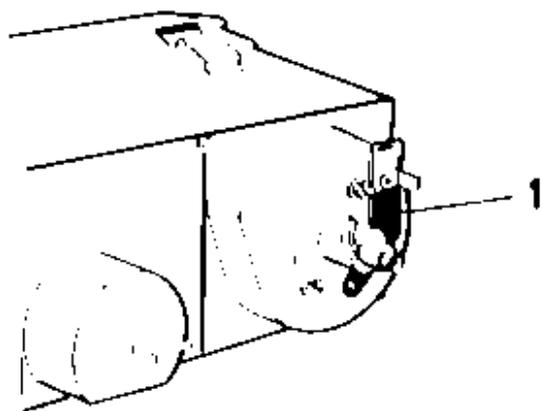
Take off the cover plate at the back of the speedometer and fit the induction transmitter (1).
