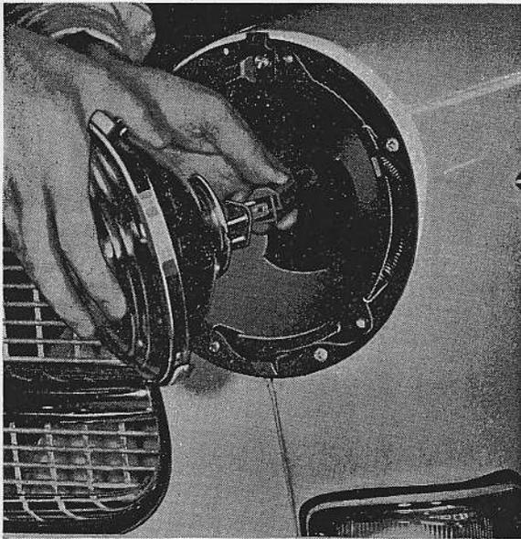
Fig. 18. Removing contact plug.
