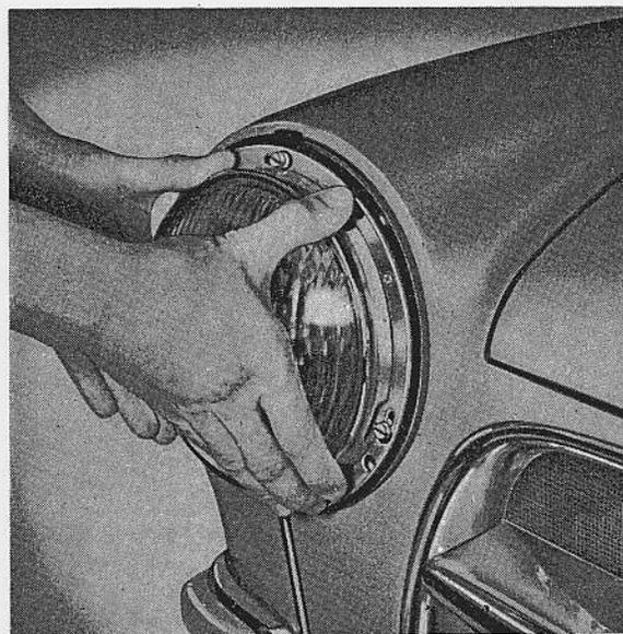
Fig. 13. Removing headlight insert.
